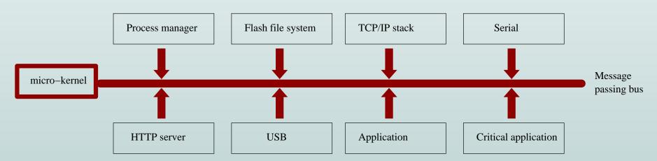
The processes communicate with each other and the hardware by means of a virtual message passing bus.
