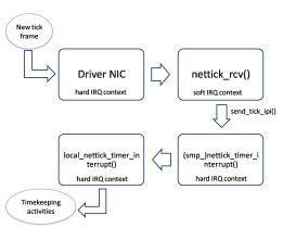
(c) From Ethernet Frame to Timer Interrupt Emulation
